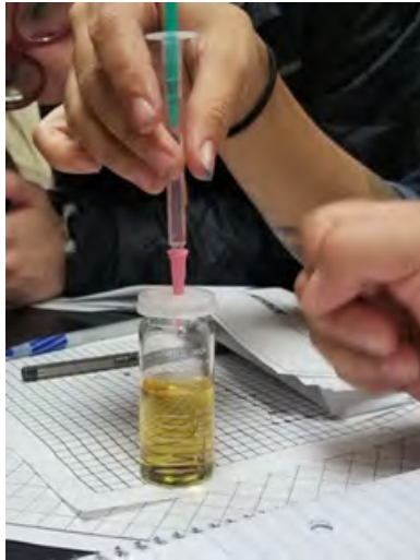
Figure 3. Number of drops of Starch indicator added to the solution until color change from yellow to colorless was measured to determine DO.
